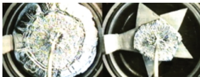
Figure 2 Deposit on circle and star shaped anode
